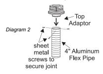
4) Pass the flex pipe down through the center of the chimney system, and center the adaptor on the top of the chimney pipe. Drill four 1/8" diameter holes through the adaptor and into the chimney top. Insure that you are in fact, drilling into the metal on the chimney. Twist-lock the Termination Cap (Part# 980 or 991) onto the Adaptor. (Diagram 3 and 4).
